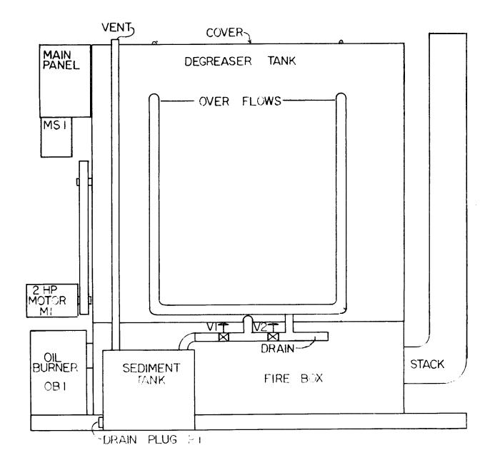
DEGREASER OIL FIRED CENTRIFUGAL IMPACT TYPE AUC-81A
